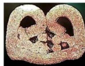
Crimp Too Loose and Void on Both Sides
