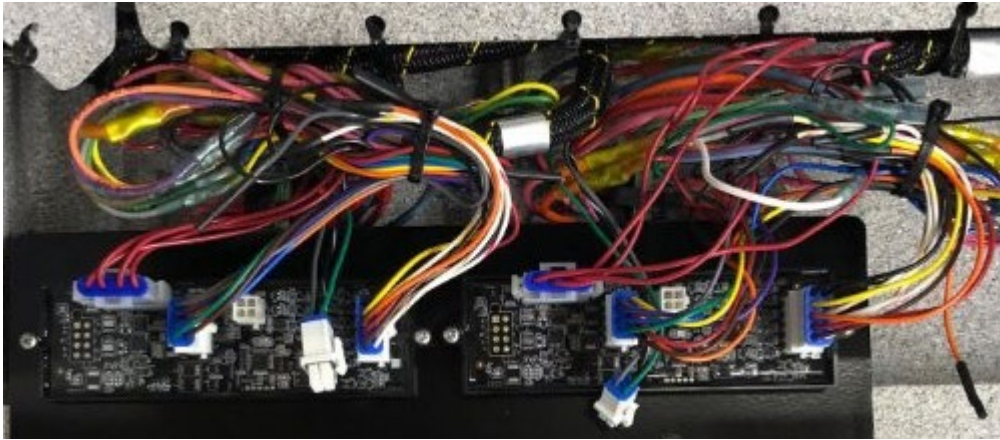
Figure 128: Example of Correct Tension on Mini Universal Mate-N-Lok Connectors
