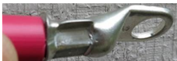
Figure 126: Example of Bad Crimp: Fins - Lug/Ring Connectors
