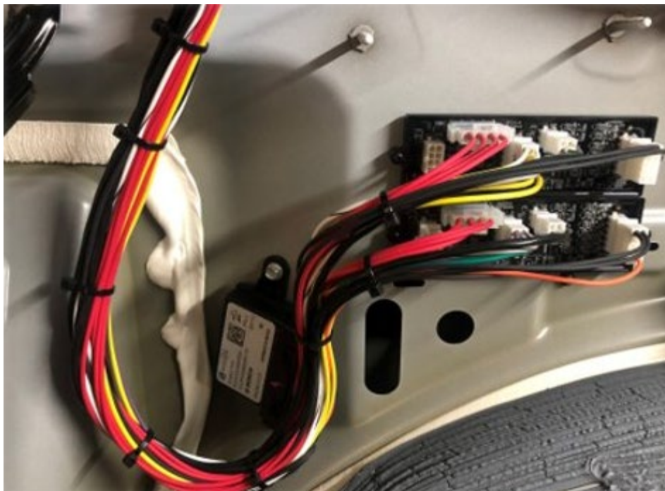
Figure 129: Example of Correct Service Loop
