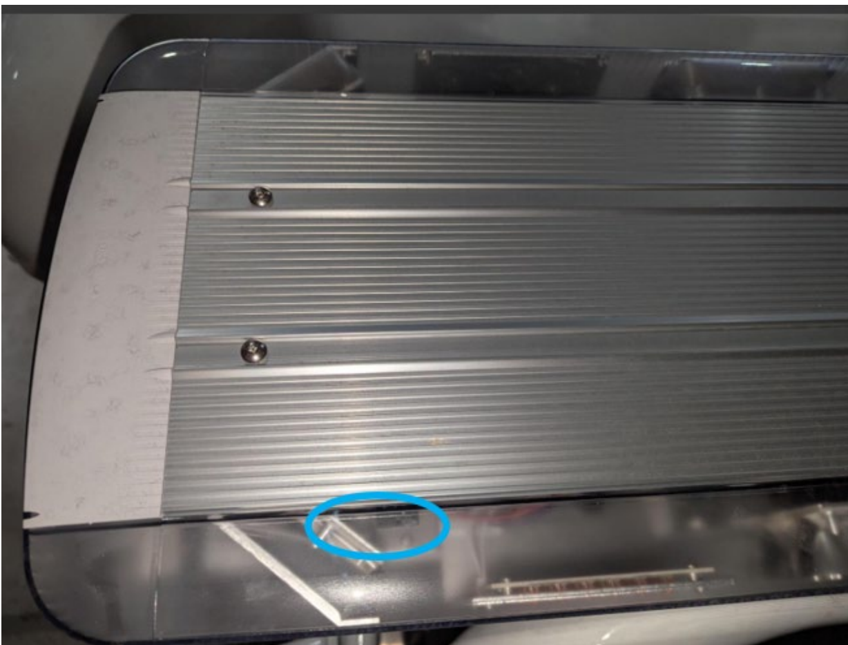
Figure 58: Photocell on Lightbar
