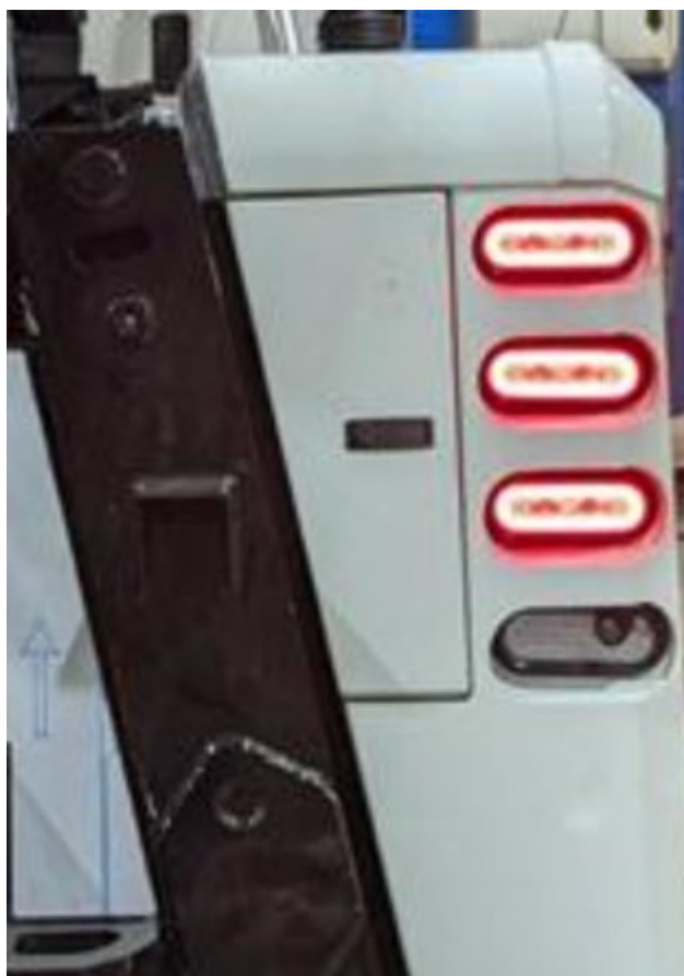
Figure 52: Paccar, Peterbilt, Kenworth Chassis: Three Marker/Brake/Turn Lights, One Reverse Light
