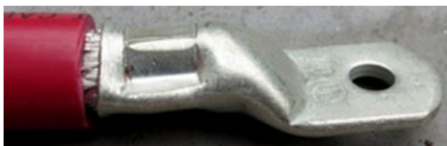
Figure 125: Example of Bad Crimp: Over-Crimping - Lug/Ring Connectors
