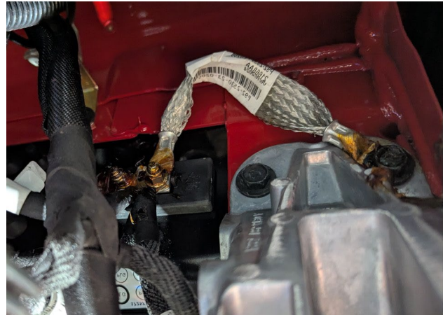
Figure 38: Example Under-Hood Ground Location
