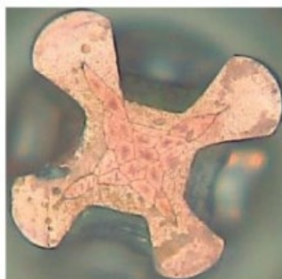
Uneven Crimp and Wall Thickness
