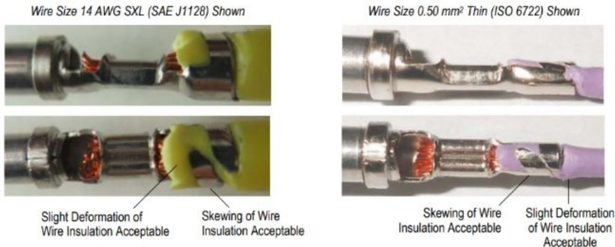
Figure 113: Examples of Acceptable Wire Crimp - Stamped & Formed Connectors
