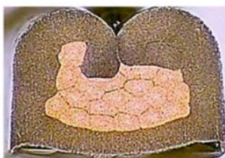
Uneven Crimp and Wall Thickness and Flash on Both Sides
